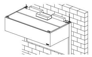
Connect the remaining ductwork for the back supply and the hood. It is recommended that caulk be applied at the mating seams and surfaces of the back supply, the hood, and the wall.
